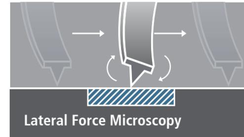
While more traditional AFM techniques focus on vertical deflections of the cantilever to image the surface topography, lateral force microscopy (LFM) instead focuses on torsional deflections as the cantilever twists as the tip is dragged across a sample surface provides useful insight into the frictional force and adhesion properties of the sample.
