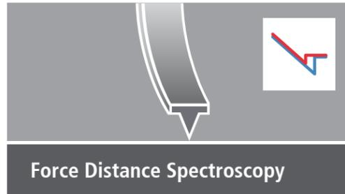
A force-distance curve is acquired by bringing the cantilever tip into contact with the sample surface. The shapes of specific regions of force-distance curves offer insight into different mechanical properties, such as adhesion, Young's modulus, etc.
