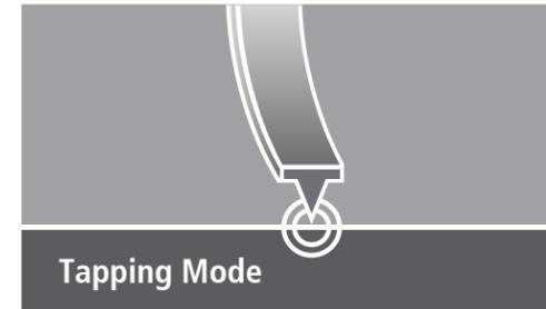
In this imaging mode, the cantilever also oscillates (as in non-contact mode) with the probe coming into intermittent contact with the sample surface. This enables improved imaging capability for certain samples whose surfaces require this type of interaction for optimal characterization.
