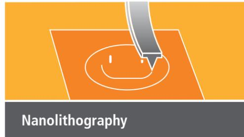
Here, the cantilever is used to intentionally modify the sample surface via mechanical and/or electrical means. To mechanically alter a surface, a specialized, robust cantilever gouges the surface with excessive force. To electrically alter a surface, a cantilever with a high bias is used to oxidize local surface regions.
