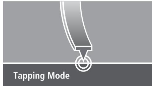
In this imaging mode, the cantilever also oscillates (as in non-contact mode) with the probe coming into intermittent contact with the sample surface. This enables improved imaging capability for certain samples whose surfaces require this type of interaction for optimal characterization (e.g., block copolymers).
