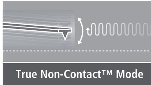
In this technique, the cantilever oscillates just above the surface as it scans. A precise, high-speed feedback loop prevents the cantilever tip from crashing into the surface, keeping the tip sharp and leaving the surface untouched. As the tip approaches the sample surface, the oscillation amplitude of the cantilever decreases. By using the feedback loop to correct for these amplitude deviations, one can generate an image of the surface topography.
