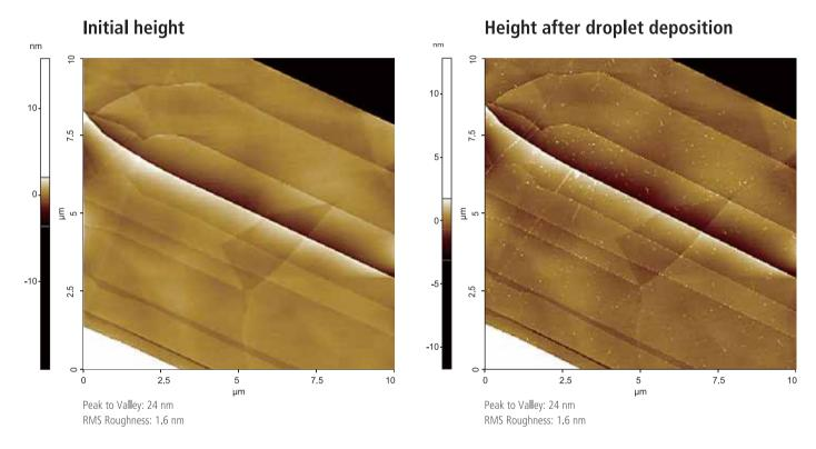
Water droplets deposited on HOPG surface were observed under humid condition in glove box.
