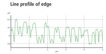
Measurement of sidewall roughness on Si line patterns by location. Despite the same semiconductor fabrication process, there is a difference in roughness between the center and the edge of the wafer.
