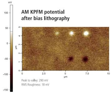
Surface potential was measured after "dots lithography" on PZT thin film.
