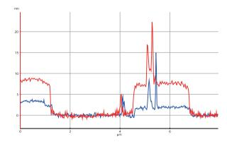
The height difference between graphene and SiO<sub>2</sub> was observed after applying 10 V to graphene surface.
