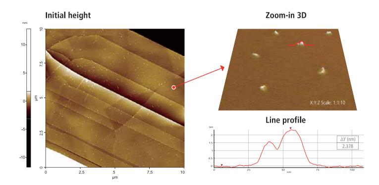
Measured water droplet height: ~2.4nm.
