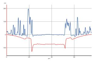
Cu via on SiC wafer. The via pattern surface changed after chemical mechanical polishing (CMP) process.
