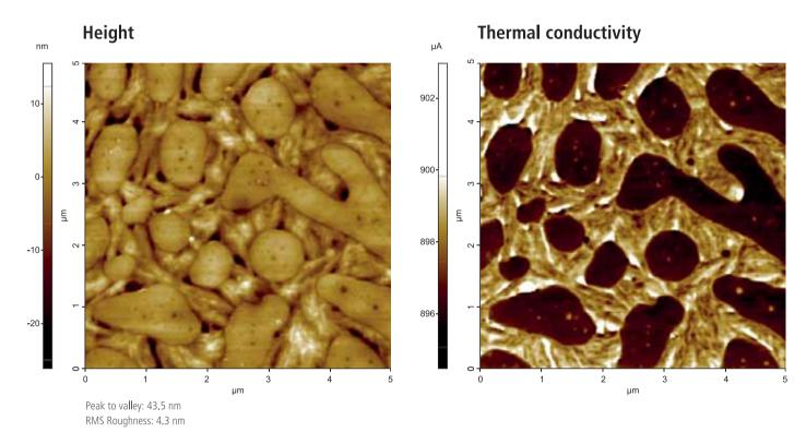
Composite of LDPS and PE. Probe current shows different thermal conductivity by materials.
