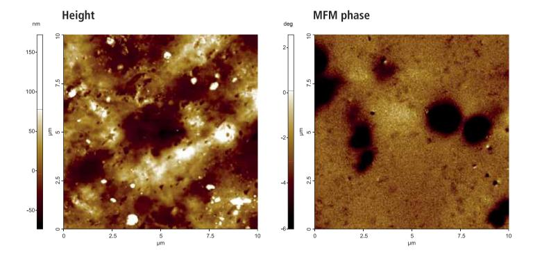
The iron particles are obviously distinguished from the rubber in MFM image.
