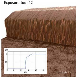
Study on the dependence of exposure tools on sidewall roughness.
