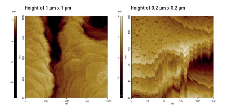
Self-assembled monolayer (SAM) on Au made from organothiols (C10) containing.
