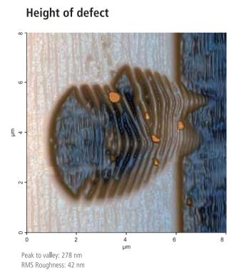
Wrinkle patterns of epitaxial SiC and defect by ion dropping after Cs+ ion gun sputtering.
