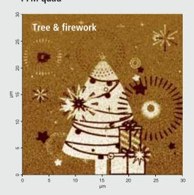
Re-arranged the domain pole direction on PZT surface using bias mode of lithography.
