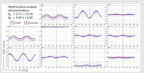
θ-spectrum of the normalized 3x4 MM of black phosphorus at different angles of incidence obtained from ROI-evaluation of MM-micromaps. Indices of fitted complex refractive indices  $N_{\alpha}$  and  $N_{\beta}$  refer to principal inplane axes of index ellipsoid (c. figure left, inset in  $m_{34}$ -micrograph). Mind different y-scales for block diagonal and block off-diagonal MM-elements.
