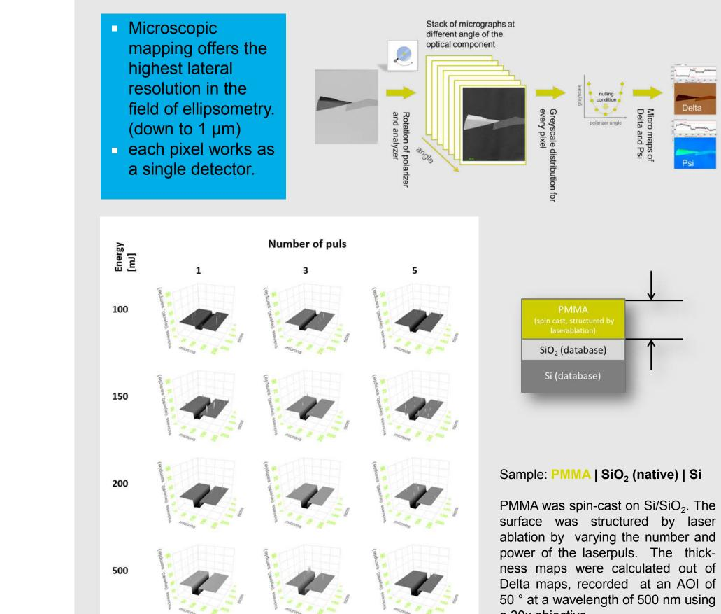
The ep4 is the latest microscopic imaging spectroscopic ellipsometer with unique measurement capabilities. It can provide real-time ellipsometric enhanced contrast images, and maps of the ellipsometric angles Psi and Delta. These data can be transferred into Thickness and the complex refractive indices by computerized optical modeling.
