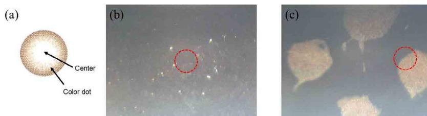
Figure 2. (a) Concept drawing of a soft contact lens with a color layer; (b) Optical camera image: Center of the lens surface on the convex top region; and, (c) color coated area. The red circles mark the AFM scan areas. The optical image scale for both (b) and (c) is  $480 \mu\text{m} \times 360 \mu\text{m}$ .
