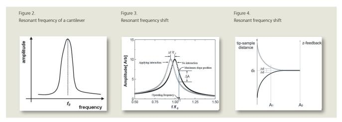
On the other hand, the spring constant affects the resonant frequency ( $f_0$ ) of the cantilever, and the relation between the spring constant ( $k_0$ ) and the resonant frequency ( $f_0$ ) in free space is shown as in Equation (2).
